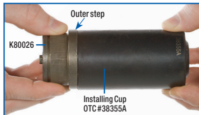
Correct fit, against outer step
