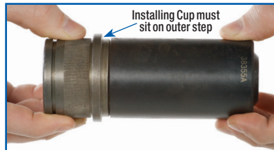
Incorrect fit, not against outer step
